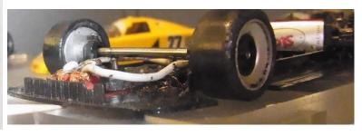
Note suspension at the rear of the motor-pod and the front axle adjustment which allows the wheels to rotate freely with just enough upwards travel to stabilise the car in the corners.
