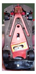
Note weight placed within the motor pod with a small amount in front of the front axle above the guide. A Slotting Plus Axle tube is used here – presumably to prevent flex although this is not common.
