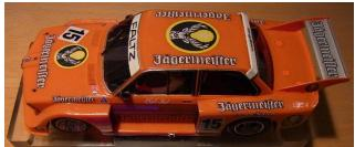
Cars are run virtually box standard with the Yellow Flat-6 AW motor and 28z / 11z gearing. Substituting a Slot.it zero offset motor pod is permitted (recommended – see left) but not imperative. Wheels and Tyres are free choice as is Guide but the one it comes with is usually fine.
