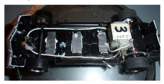
▲The optimum set-up; Rear track should ideally be 60 mm and the overall weight circa 86 gms with the chassis as above weighing 55 gms±
