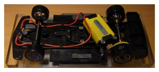
▲ This BMW 320 was set up by me – the front weights would probably be better centrally under the front axle whilst using a Slot.it motor mount would allow the side ones to be placed on the mount ahead of the motor.
