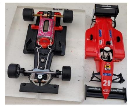
tyres (the rears being particularly critical) and a degree of motor and body float, and setting up the front axle height to allow a little upward travel in the corners the main changes from standard are the use of;
