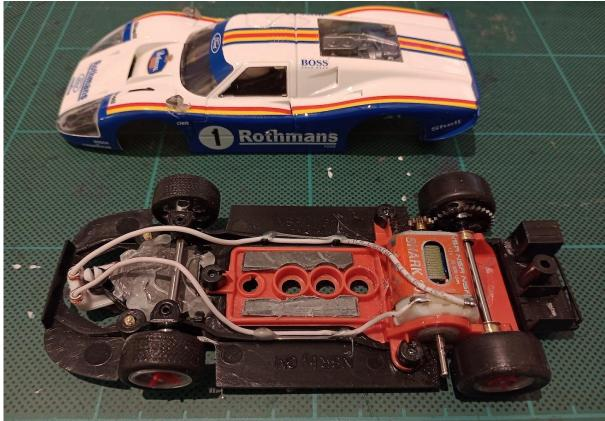
These cars are run pretty much as they come out of the box – the only changes permitted are adding weight / glueing and trueing the tyres (including coating the fronts with Nail Varnish or Superglue) and substituting the body screws for Metric type. Tyre size must be correct for the car. Wheel Inserts should be fitted and the standard Racing Pickup guide (NSR Part No. 4841) must remain as supplied.
