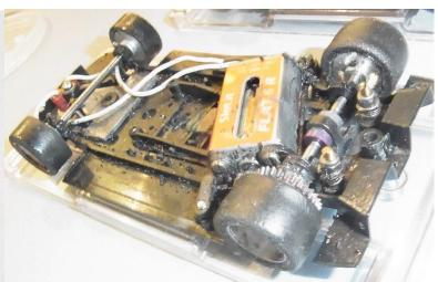
NB. NSR braids and silicone motor wire are used together with Slotting Plus axle stoppers at rear.
